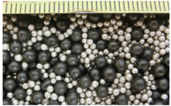
Fig. 7. Photograph of material M3, glass beads mixture.
